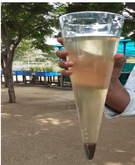
Floc volume measurement with Imhoff cone
