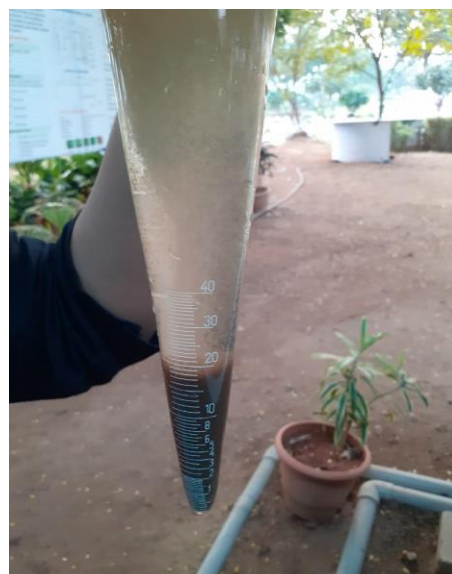
Floc volume measurement with Imhoff cone
